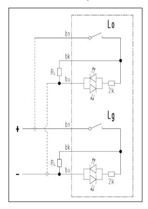
12.....30V Operating voltage range AC / DC (=Vb) ±10% Vb Max. permitted residual ripple Max. permitted switching current 500 mA
