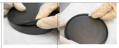
Remove the gate gliders from the valve gate with a little tool e.g. screwdriver.
