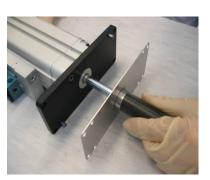
Before mounting the new bellows feedthrough be aware about the flat encoding sections on the actuator shaft. This flat encoding section should orientate the valve gate later on.
