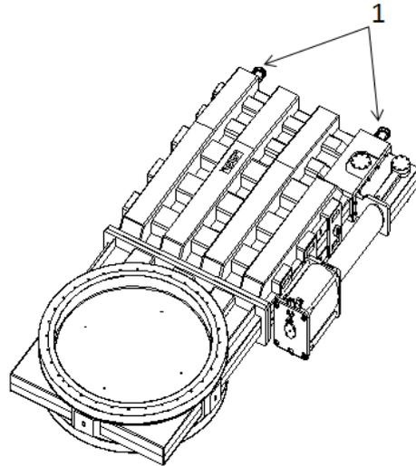
1 Load rings for valve lifting
