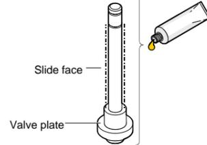
... and wipe the flange and valve plate seals with a lint-free cloth moistened with high vacuum oil (583413).
