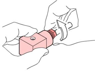
10 Remove the clamp and turn the solenoid coil so that the electrical connection is in the desired position. Fix it by inserting the clamp.
