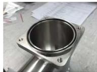
3. Insert bellows feedthrough (15) carefully
