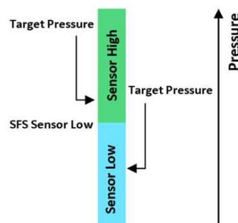
If target pressure is in the range of low sensor, low sensor is used; otherwise high range sensor.
