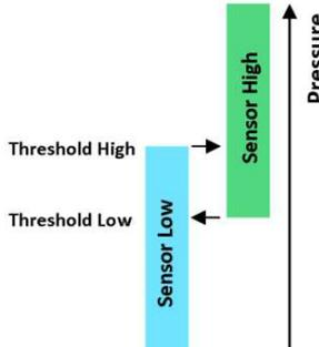
Switching between sensors according to the hysteresis threshold levels and an optional delay.
