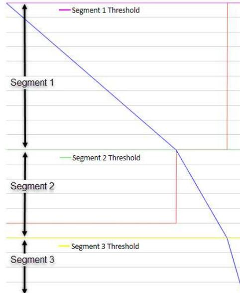
**Segment x Slope** Defines the slope (pressure/sec) in the segment
