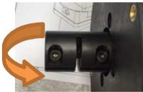
7. Insert the coupling of controller (26) on rod (2) until it stops and tighten the coupling screw (12) with a torque of 2.2 Nm
