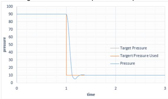
New Target Pressure with pressure ramp
