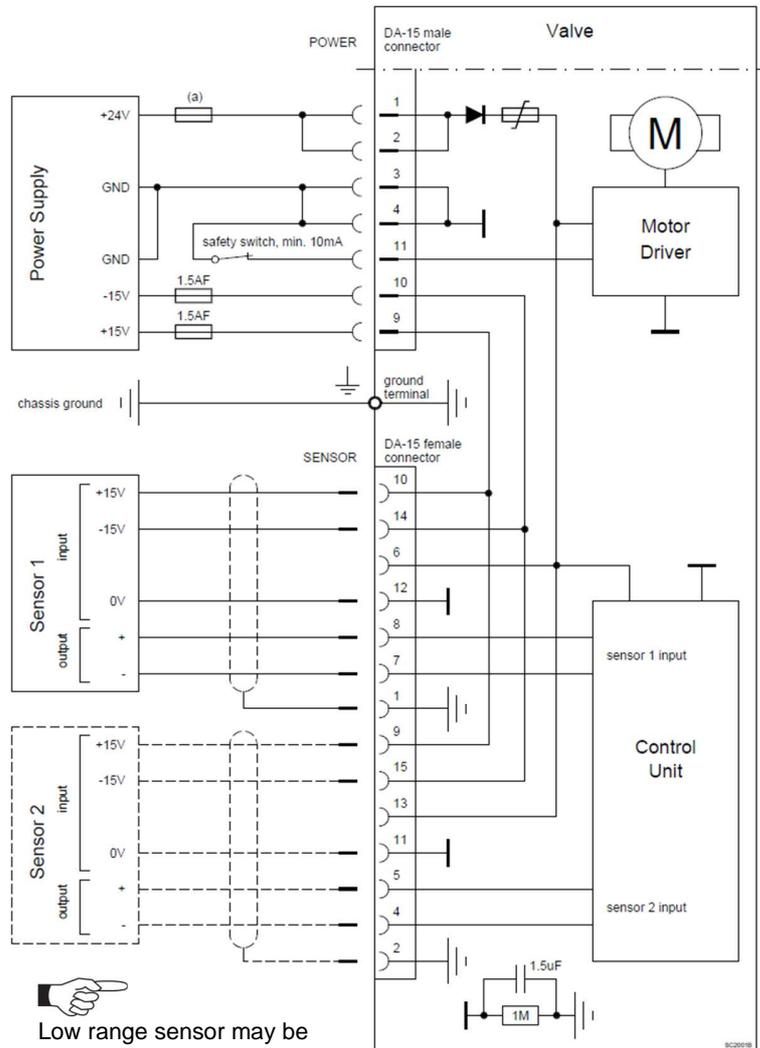
Pins 4 and 11 must be bridged for operation. An optional switch would allow for motor interlock to prevent valve from moving.
