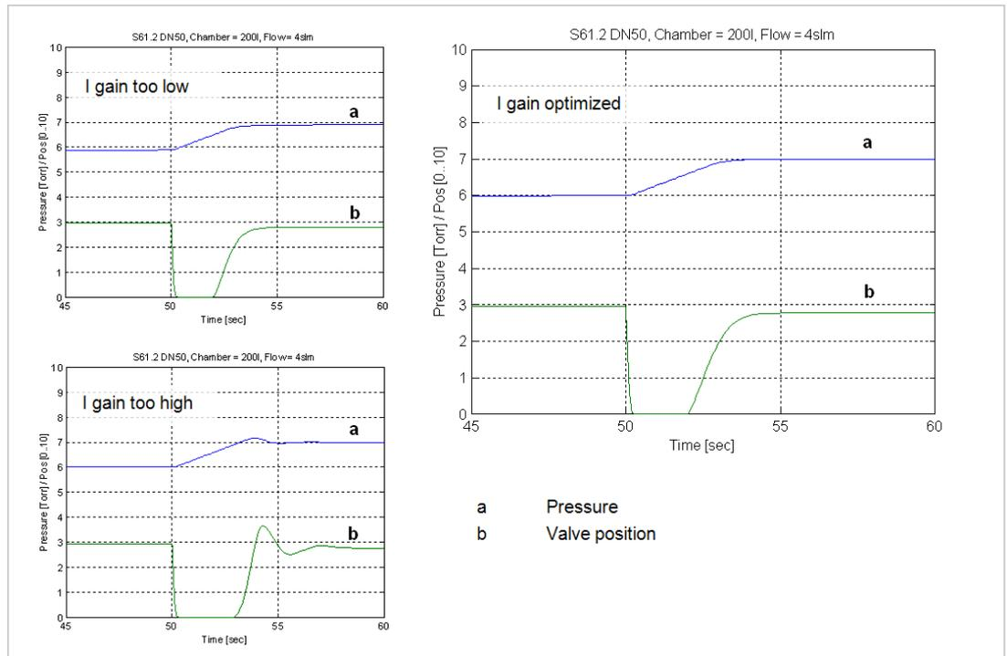
Check control performance over the whole control range with parameters above.
