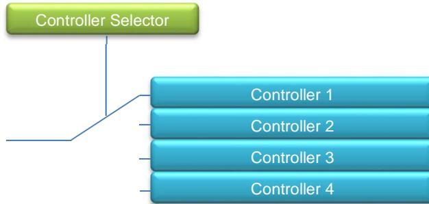
Most applications do not need more than one controller unit. But if the result of the pressure control does not meet the expectations, the different controller units can be an option for optimization: With the four controller units it's possible to use an own controller unit for a specific pressure working point. This controller unit can be parametrized optimally for this specific working point.
