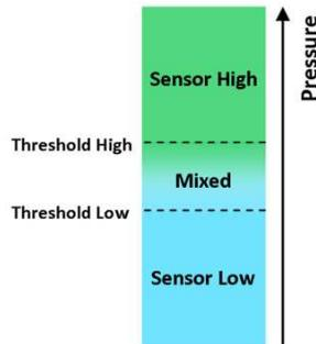
Within the threshold levels, the resulting measurement value is a summation of the two sensors signals with a proportional ratio of the two measured values.
