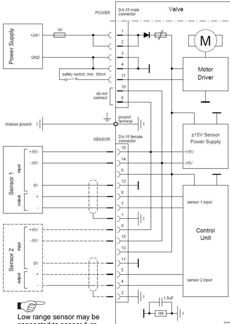
Pins 4 and 11 must be bridged for operation. An optional switch would allow for motor interlock to prevent valve from moving.
