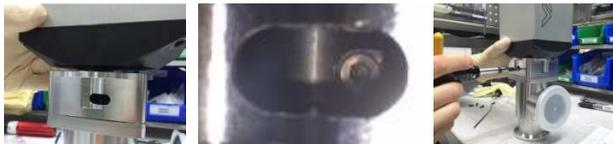
8. Turn controller over stop (flange) and on the right position (see drawing), and fasten the actuator screws (59) uniformly and in crosswise order with a torque of torque 3 Nm
